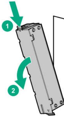
10. Install the optical drive bracket.
