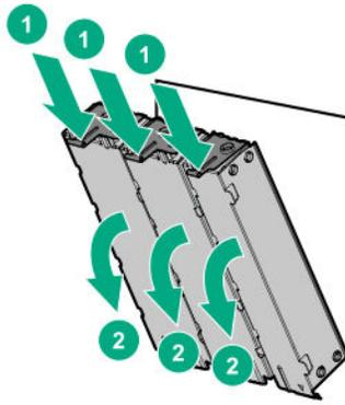
If the drive cage is to be installed in box 2 or 3, remove the drive cage blank.
