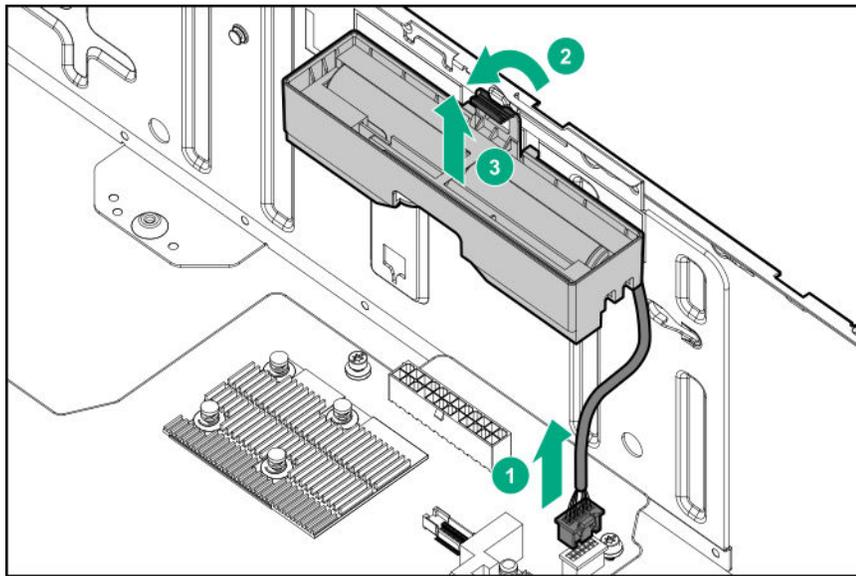
11. Disconnect the non-hot-plug power supply cable.
