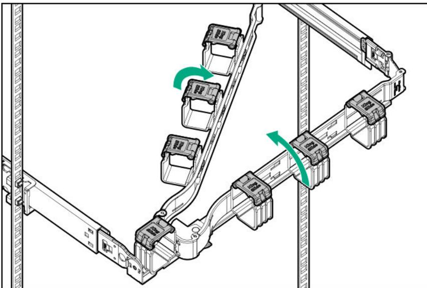
4. Route the rear panel cables and power cords through the CMA, and then close the cable clamps.
