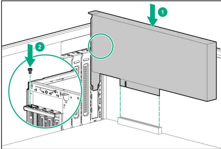
17. Make sure that the boards are firmly seated in the slots.
