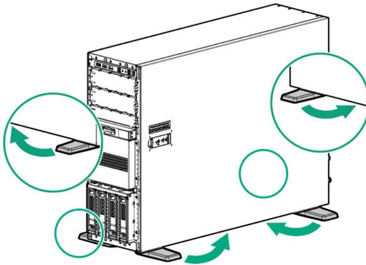
2. Place the server on a flat, level surface with the access panel facing up.
