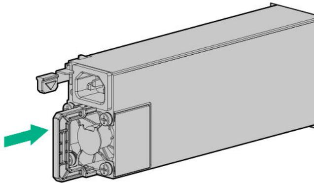
3. Connect the power cord to the power supply.
