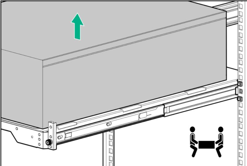
8. Place the server on a flat, level surface with access panel facing up.
