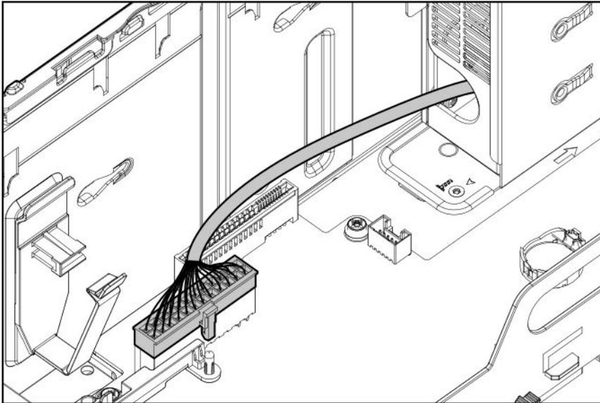
**12.** Remove the non-hot-plug power supply.
