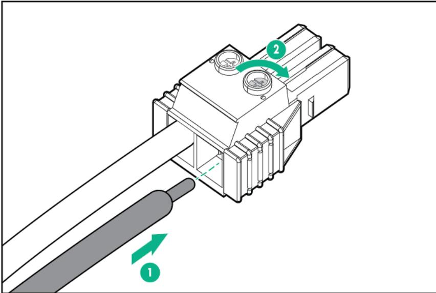
9. Install the terminal block connector in the power supply.
