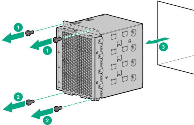
10. Remove the spare screws from the drive cage.
