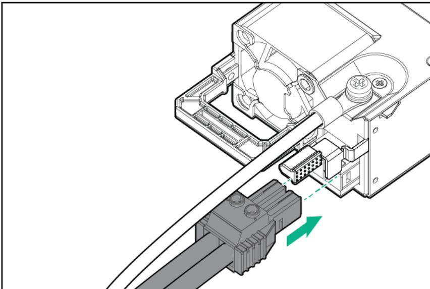
10. Secure the power cord, wires, and cables in the strain relief strap attached to the power supply handle:
