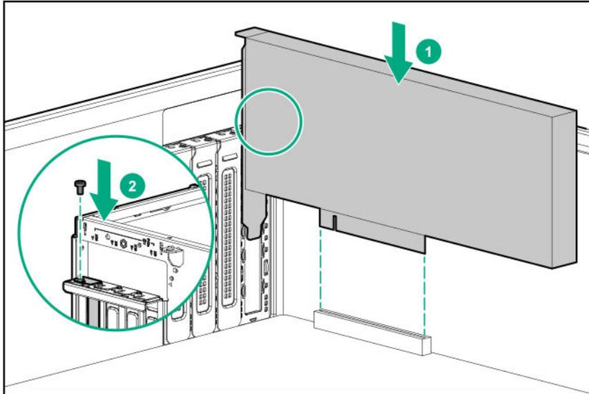
14. Make sure that the board is firmly seated in the slot.
