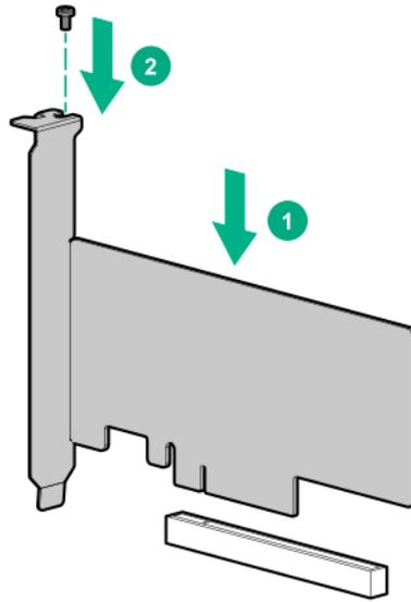
**14.** Make sure that the board is firmly seated in the slot.
