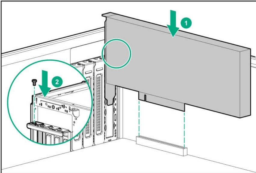
15. Make sure that the card is firmly seated in the slot.
